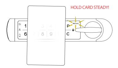
ACCIDENTALLY TOUCHING A DIGIT KEY WHEN PRESENTING A PROX CARD, CAN DELAY READING OF A CARD.
